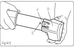
To remove tool: Push forward and up on tab (F). Slide tool off hose wand.
